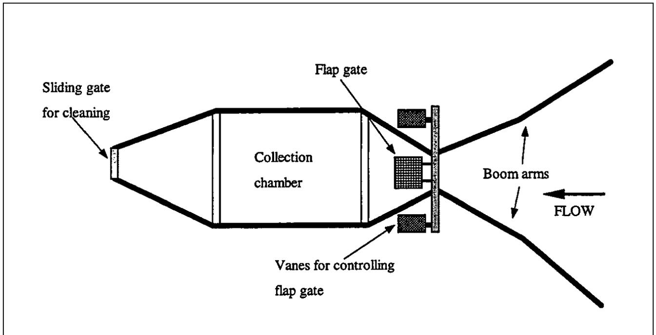
Figure 6: Plan view of Bandalong floating debris trap
